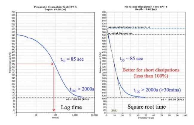
**Figure 18** Example dissipation test to determine  $t_{50}$
