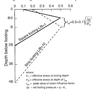
**Figure 37** Strain influence method for footings on sand (Schmertmann, 1970)
