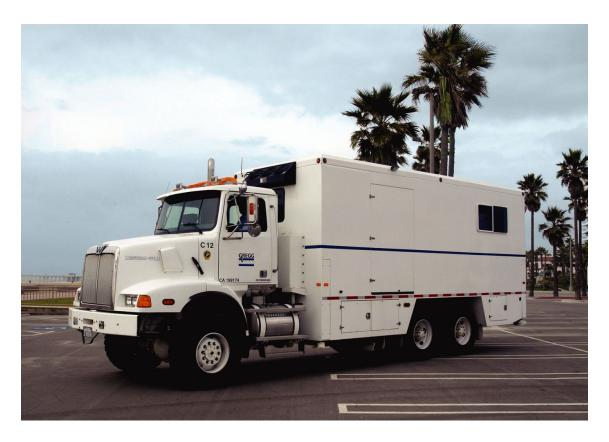
Figure 10 Truck mounted 25 ton CPT unit
