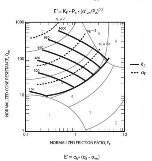
**Figure 31** Evaluation of drained Young's modulus (at ~ 0.1% strain) from CPT for young, uncemented silica sands,  $E = \alpha_E(q_t - \sigma_{vo})$  where:  $\alpha_E = 0.015 \left[10^{(0.55Ic + 1.68)}\right]$
