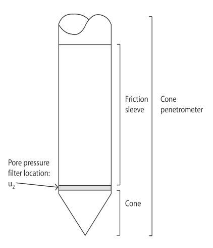
Figure 2 Terminology for cone penetrometers
