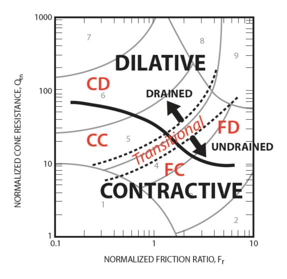
**Figure 26** Normalized CPT Soil Behavior Type (SBT<sub>n</sub>) chart, Q<sub>t</sub> - F using general large strain 'soil behavior' descriptors (Modified from Robertson, 2012)
