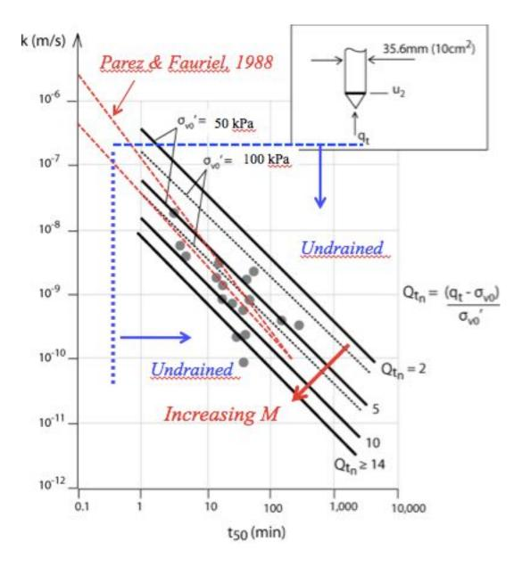
**Figure 34** Relationship between CPTu  $t_{50}$  (in minutes), based on  $u_2$  pore pressure sensor location and  $10 \text{cm}^2$  cone, and soil permeability ( $k_h$ ) as a function of normalized cone resistance,  $Q_{tn}$  (after Robertson 2010)
