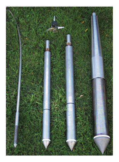
Figure 8 Range of CPT probes (from left: 2 cm<sup>2</sup>, 10 cm<sup>2</sup>, 15 cm<sup>2</sup>, 40 cm<sup>2</sup>)
