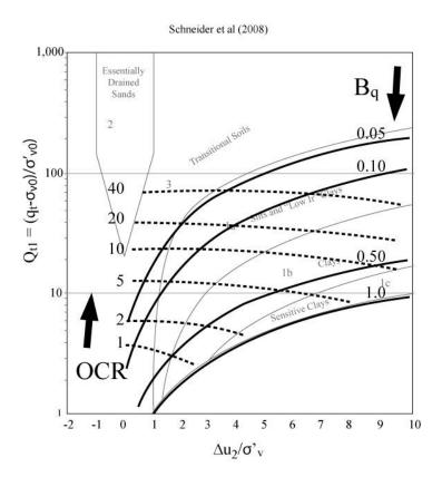
**Figure 24** CPT classification chart from Schneider et al (2008) based on  $(\Delta u_2/\sigma'_{vo})$  with contours of  $B_q$  and OCR
