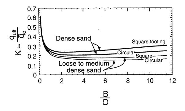
**Figure 36** Correlation between bearing capacity of footing on cohesionless soils and average cone resistance (after Eslaamizaad and Robertson, 1996)
