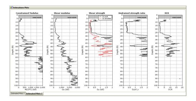
Figure 54 Example of estimated geotechnical parameters from *CPeT-IT*
