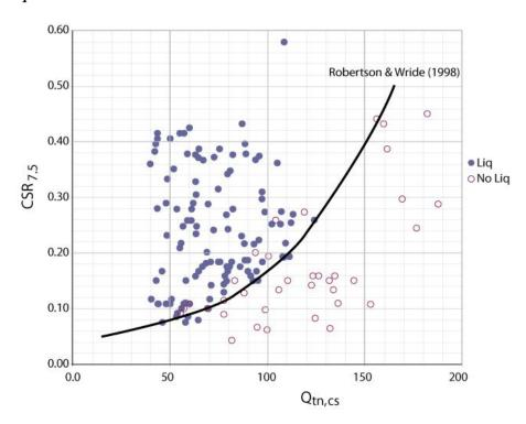
**Figure 45** Cyclic resistance ratio (CRR<sub>7.5</sub>) from CPT normalized clean sand equivalent cone resistance ( $Q_{tn,cs}$ ) (updated by Robertson, 2009)
