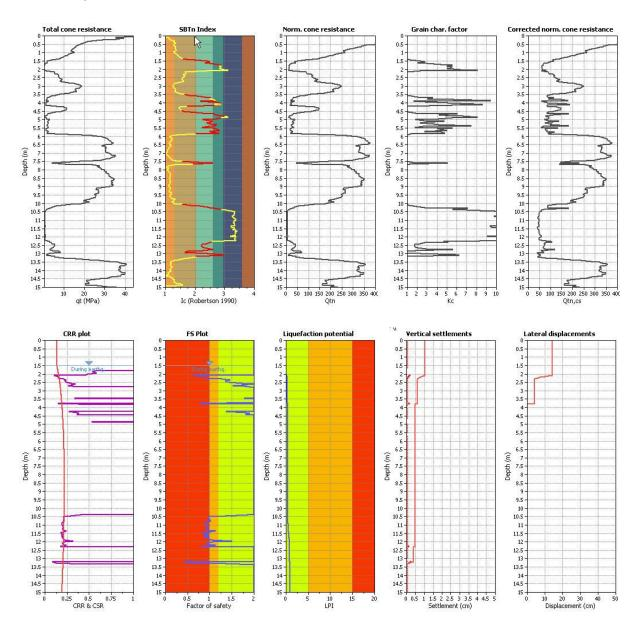
**Figure 47** Example of CPT-based approach to evaluate cyclic liquefaction/softening at Moss Landing Site showing (a) intermediate parameters (b) CRR, FS and post-earthquake deformations using '*CLiq*' software (http://www.geologismiki.gr/)
