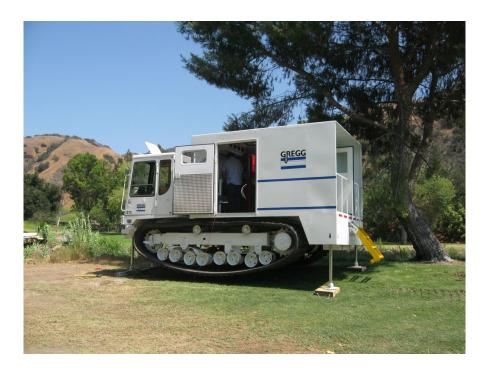
Figure 11 Track mounted 20 ton CPT unit
