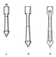
Figure 5 Dutch mechanical cone penetrometer with conical mantle
