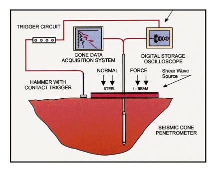
Figure 9 Schematic of Seismic CPT (SCPT) test procedure
