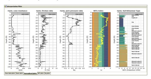
Figure 53 Example CPTu plot based on normalized parameters from *CPeT-IT*
