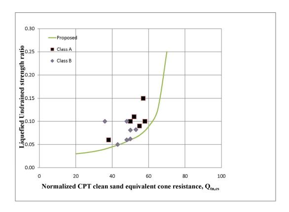
**Figure 50** Liquefied shear strength ratio and normalized CPT clean sand equivalent penetration resistance from flow liquefaction failure case histories (after, Robertson, 2010)
