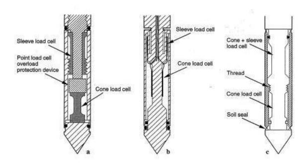
**Figure 19** Designs for cone penetrometers (a) tip and sleeve friction load cells in compression, (b) tip load cell in compression and sleeve friction load cell in tension, (c) subtraction type load cell design (after Lunne et al., 1997)
