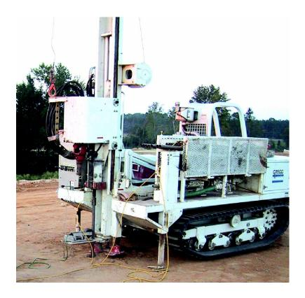
Figure 12 Small anchored drill-rig unit
